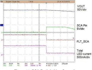
Figure 29. SCA Fault in Live Operation
