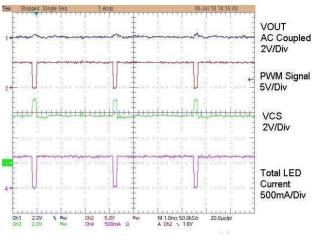
Figure 23. PWM Waveforms 95% Duty Cycle
