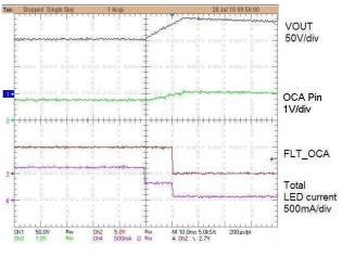
Figure 27. OCA Fault in Live Operation
