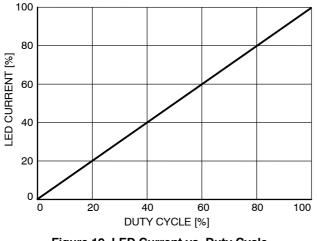
Figure 19. LED Current vs. Duty Cycle
