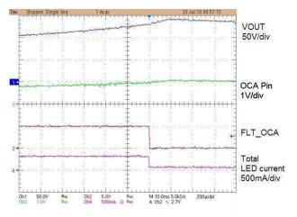
Figure 26. OCA Fault During Power Up
