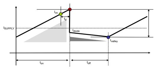
Figure 7. Tapped Coil Boost Current in the Coil
