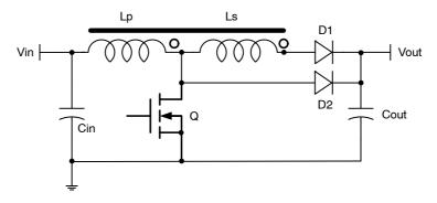
Figure 6. Tapped Coil Boost Solution Schematic
