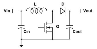
Figure 4. Conventional Boost Solution Schematic
