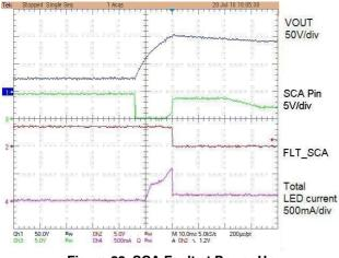
Figure 28. SCA Fault at Power Up
